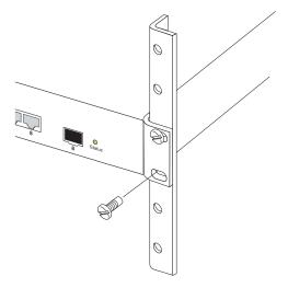
Figure 3-3 Installing the Switch in a Rack
